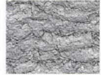
CSP 9 (heavy scarification)
